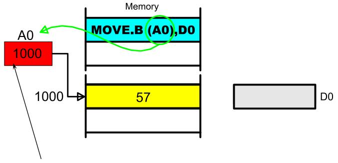
The address register in the instruction specifies an address register that holds the address of the operand
