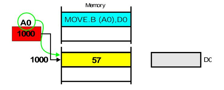
The address register is used to access the operand in memory
