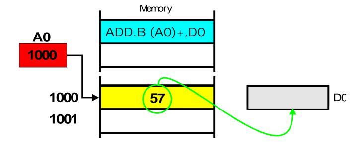
Address A0 register is used to access memory location 1000 and the contents of this location (i.e., 57) are added to D0
