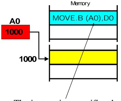
This instruction means load D0 with the contents of the location pointed at by address register A0
