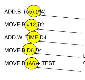
Address register indirect addressing. The address of the source operand in in A5.
