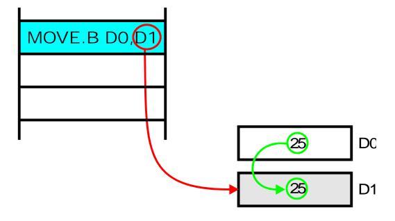
The effect of this instruction is to copy the contents of data register D0 in to data register D1
