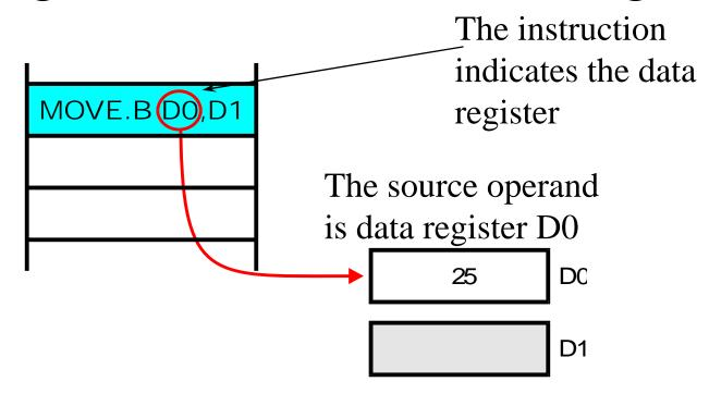
The MOVE.B D0,D1 instruction uses data registers for both source and destination operands
