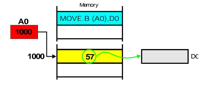
Finally, the contents of the address register pointed at by A0 are copied to the data register
