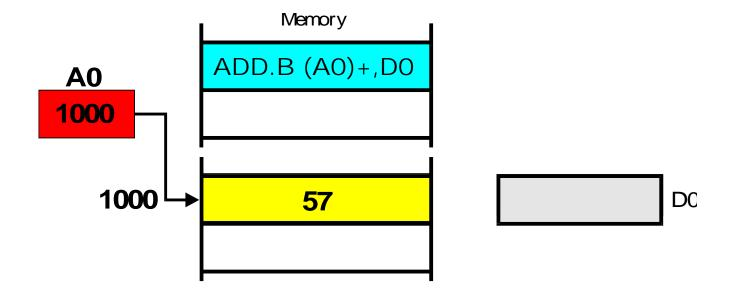
The address register contains 1000 and points at location 1000
